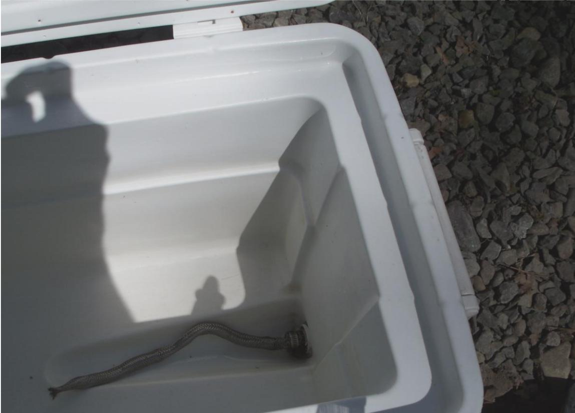
Inside of stainless steel tubing forced over a 3/8 inch ratchet piece that was set into drain of cooler by heating it up and melting it in place.
